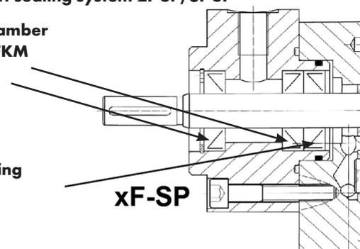
Standard inlet pressure  $p_1$ : 7 bar (in certain special solutions up to 50 bar!) Before start-up the block chamber must be filled with fluid. **Beinlich Pump Systems** recommends using Mesamoll® oil or another inert medium which does not react with the pumped fluid and which is environmentally inert should it leak. The block chamber is formed by the seal housing or by attaching a drip-feed lubricator. This is achieved by:
