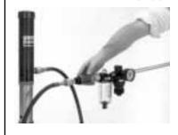
Pump "runaway" results when your material container is depleted and the pump cycles fast and needlessly. It's not good for a pump. So protect your pump investment - with an ARO-STOP® Valve.
